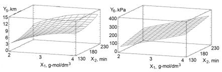
Figure 3 – Dependence of the resistance of cellulose to tearing  $Y_5$  and bursting shear  $Y_6$  on variable cooking factors
