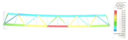
Fig. 3. N forces in elements obtained in the Midas Civil PC
