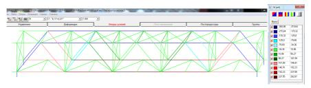
Fig. 3. N forces in elements obtained in StructureCad PC
