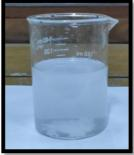
Fig.2. Dissolution of (Mg(NO<sub>3</sub>)<sub>2</sub>.6H<sub>2</sub>O) and (NaOH) in DI water
