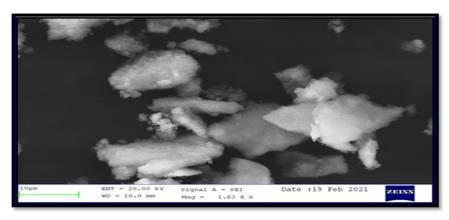
Fig.8. SEM images of MgO Nanoparticles
